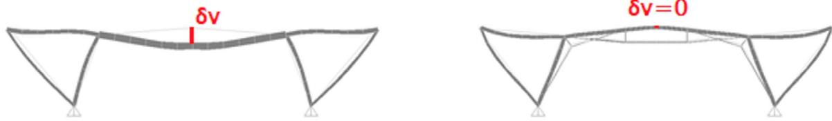
Figure 7. Comparison of vertical deflections for models A & B.
