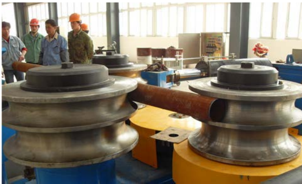
Figura 31. Curvado de tubos Figure 31. Tube curving
